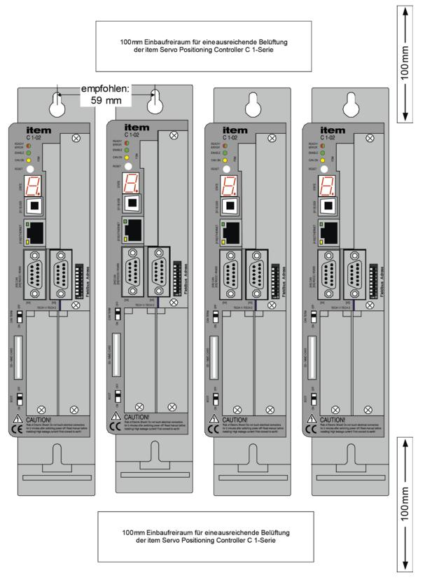
Figure 10: item servo positioning controller C 1-Series: Installation space
