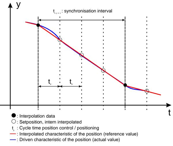
Figure 7: Linear interpolation between two data values
