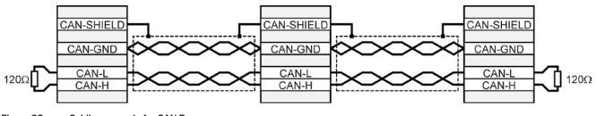
Figure 22: Cabling example for CAN-Bus
