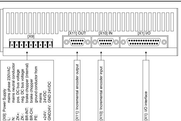
Figure 12: item servo positioning controller C 1-02: Top view
