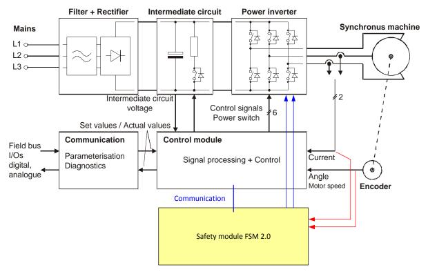
Figure 8: Schematic representation of the integrated safety technology
