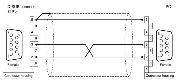
Figure 24: Pin assignment: RS232 null modem cable [X5]
