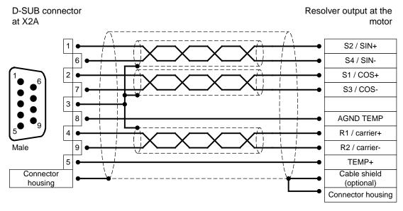
Figure 21: Pin assignment: Resolver connection [X2A]
