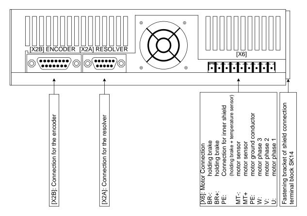
Figure 13: item servo positioning controller C 1-02: Bottom view
