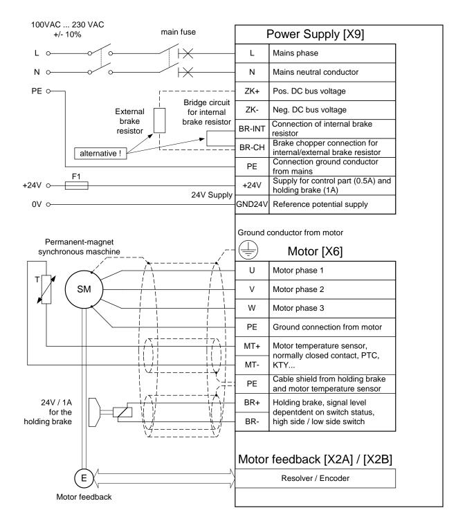
The operation of the item servo positioning controller C 1-Series requires a 24V voltage supply source for the electronics supply, which is connected to the terminals +24V and GND24V.
