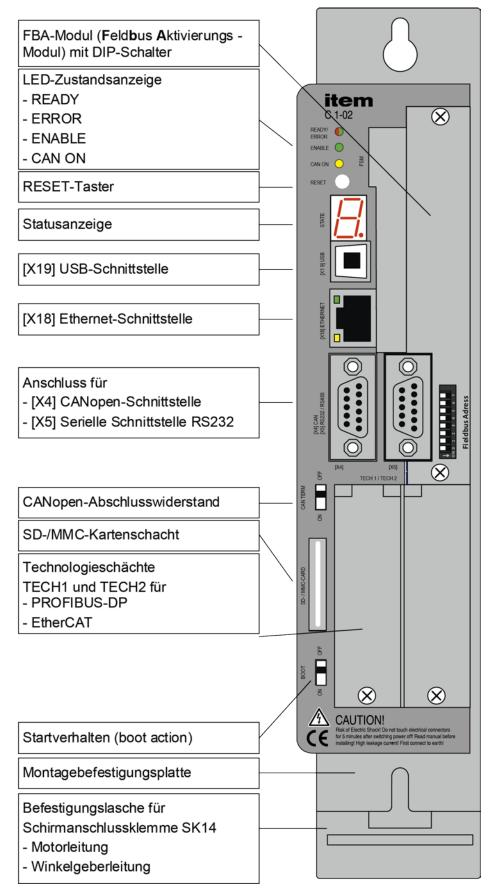
Figure 11: item servo positioning controller C 1-02: Front view
