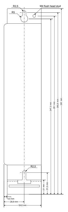
Figure 14: item servo positioning controller C 1-Series: Mounting plate
