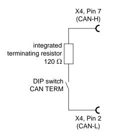
Figure 23: Integrated CAN terminating resistor
